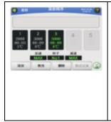
It is of vital importance to conduct test through programs which can reproduce user experimental package by calling out the program number. Five centrifugal stages can be set to satisfy your demand for diversified experiments. One button to start your perfect experimental package (100 programs are built-in and each program is divided into 5 steps, and more programs can be set with external memory )
